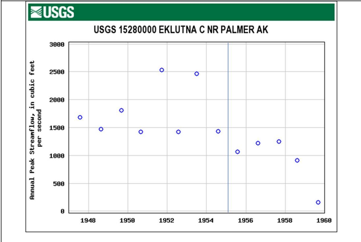
While typical pre-1955 seasonal streamflow ranged from approximately 100 cubic feet per second (cfs) to as much as 1,000 cfs, recent streamflow measurements on the Eklutna River downstream from the lake outlet, excluding rare spill events, have averaged 8 cfs with a maximum measured flow of 24 cfs.
